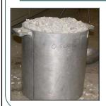
Percent Voids in a compacted sample of Coarse Aggregate. Expressed as a decimal (0.XX)
